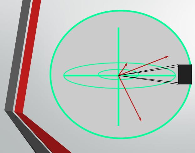
As the distance from the sound source increases, the area covered by the sound wave increases.
