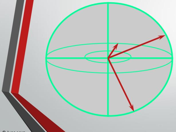
• Sound waves propagate spherically, or omnidirectionally.
