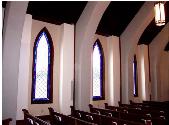
Pastor Jon Schroeder states: The interior design of our sanctuary could be called neo-gothic. Specifically, it emphasizes verticality, and utilizes load-bearing masonry. The nave is built on four 50,000 pound concrete arches. They serve both functionally to support the roof, and aesthetically to give the space a sense of rock-solid stability. The verticality of the space and upward sweep of the windows help to communicate that we are in the house of God; we have come to worship He Who is Above.
