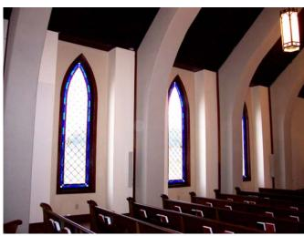
Pastor Jon Schroeder states: The interior design of our sanctuary could be called neo-gothic. Specifically, it emphasizes verticality, and utilizes load-bearing masonry. The nave is built on four 50,000 pound concrete arches. They serve both functionally to support the roof, and aesthetically to give the space a sense of rock-solid stability. The verticality of the space and upward sweep of the windows help to communicate that we are in the house of God; we have come to worship He Who is Above.
